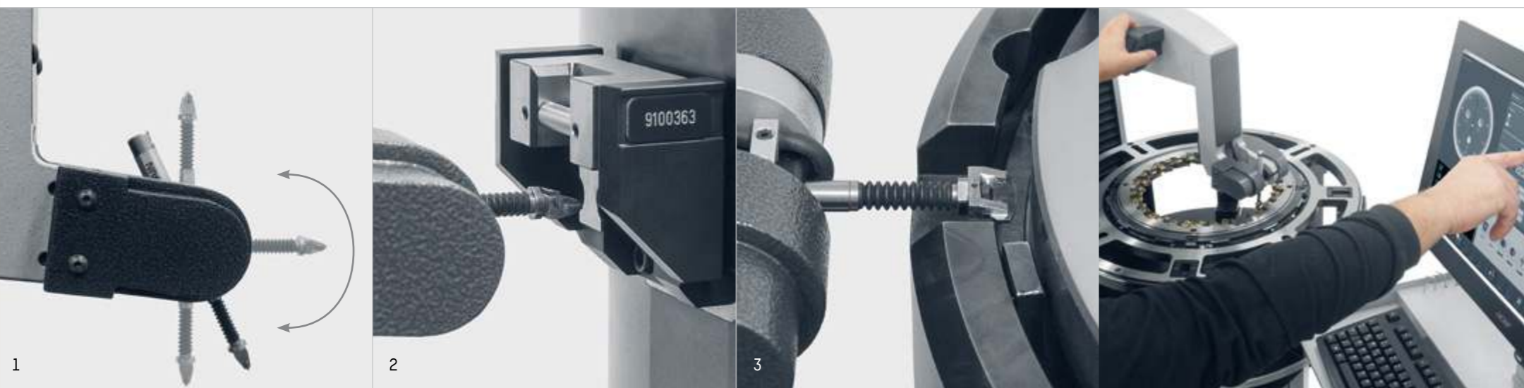
On the »aralon« the crankshaft cutter is automatically positioned accurately in the tool holder via the quick-change holding fixture. The centering collet is designed tool-specific.
