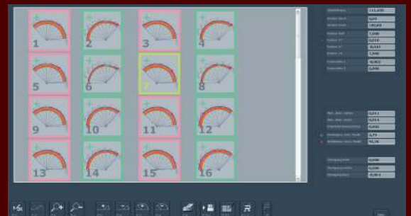
Graphical evaluation of the flanging radii (top hat).
