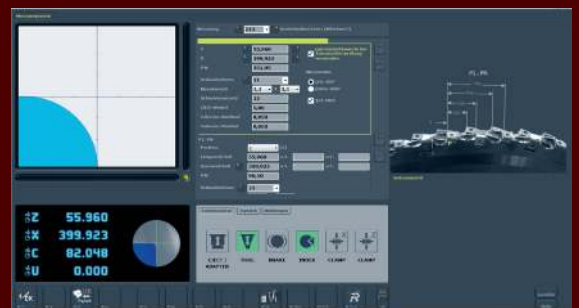
Measuring program for calculating the average values of circumferential cutting edges at several cutting edge stages.
