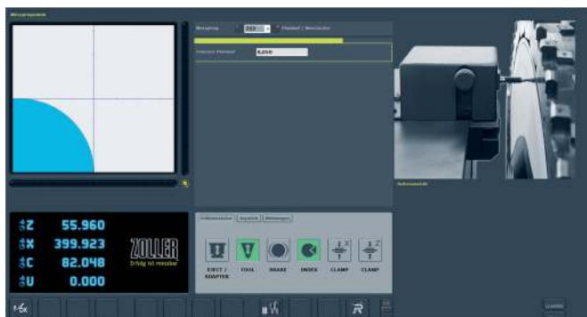
Automatic axial run-out compensation
