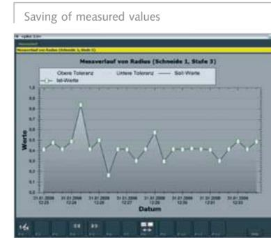
The measured values of saved tools are recorded automatically with each measurement, can be evaluated statistically and called up at any time.
