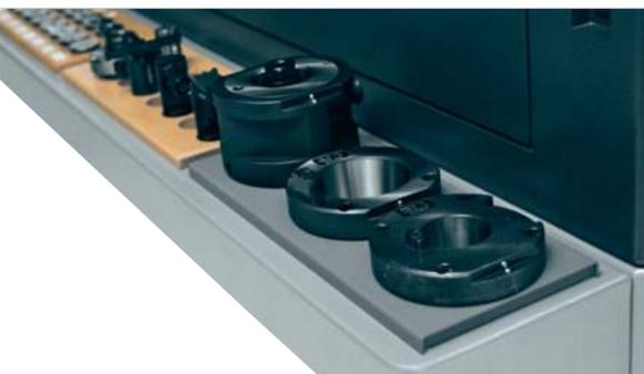
Space-saving and easily accessible trays for accessories such as changeable sleeves, adapters and tool posts.
