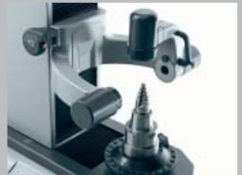
In the axial position for measuring the face on drilling and milling tools.
