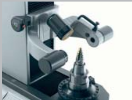
In any position for measuring along the plumb line on chamfers and corner radii.
