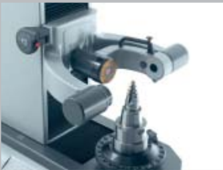
In the radial position for measuring in incident light on the circumference.
